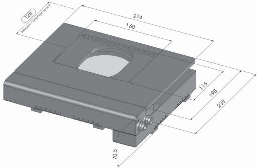
Scanning Stage SCAN 100 x 100 for upright microscopes
